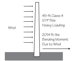
The bending moment due to wind can be calculated using the following equation. An example problem is used to illustrate the process for a 45'-4 SYP pole in NESC heavy loading.
